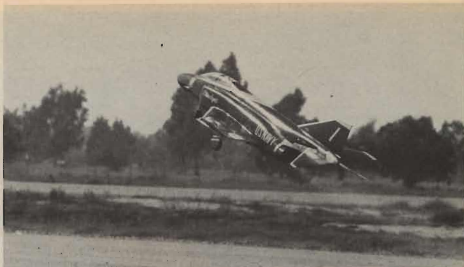
Talk about jet-like performance, Tom Cook's F-4 was a rocket with its twin ducted fans. The model weighed 17 lbs.
