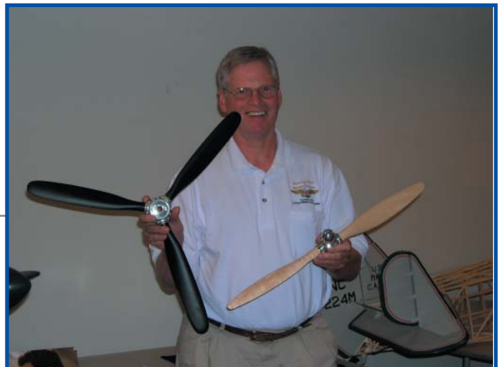
Gary Holderness holds two scale propellers with ground adjustable pitch. The left prop is for a Hellcat and the prop on the right is for a Piper Cub. I didn't catch the name, but these are really scale.
