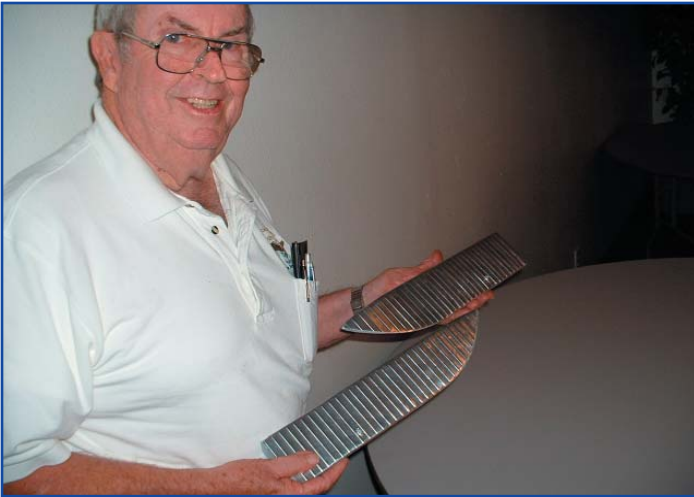
Bob Richards with scale ailerons for his WACO Bi-plane project. Made from disposable this aluminum cookie sheets.
