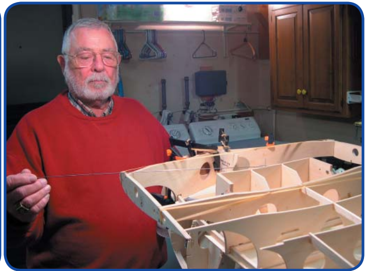
Rich Koehrer using a wire to square off the cabin frame on the big Zirolli Staggerwing. Rich and Sam teamed up on this one and Rich is the master builder on the project. Sam is handling the electronics, Stits covering and paint.
