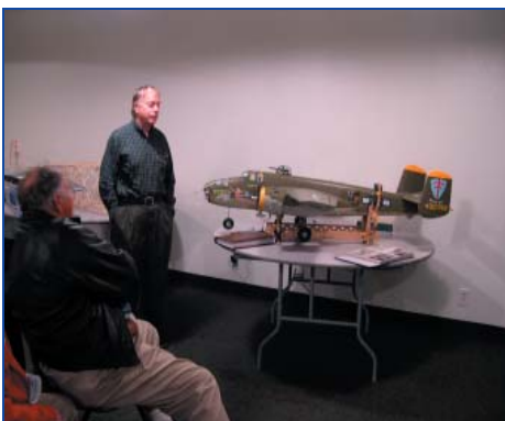
George Peter's 16 lb KMP Electric Heavenly Body B-25. Has lights, 10 bombs & 2 AXI 4120 motors.
