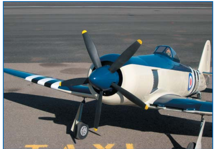
Chris Wolfe's Thunder Tiger Sea Fury at Miramar with his 5-blade scale prop. Powered by a Neu Motor and twin 6000 MAH Lipo packs. Flew really well.
