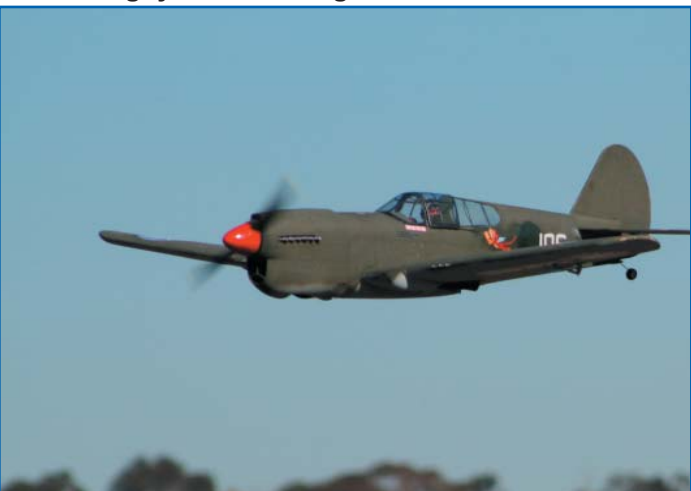
The Chino P-40 on a fly by...no, Sam Wright's Kyosho P-40 on a Hacker B50 gear drive and 5000 parallel Lipo Pack. Photo at the Miramar Field. Sam at the controls!
