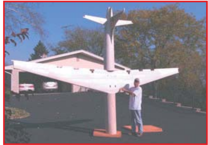
Carl Bachuber of Maryville, Wisconsin and his 1" to the foot B-36 with a 19.3' wingspan. Powered with 6 Zenoah G23's with prop extensions and 4 electric ducted fans. Prop shafts and special gear are by Bob Walker of Robart.
