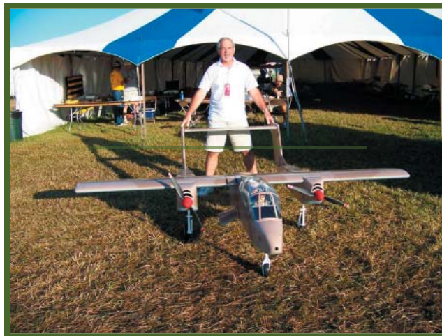
Rich Uravitch's latest Scale ship, the OV-10 Bronco. This is 22.5% scale at a 108" wingspan & powered with two Hacker A-60 Brushless Motors. All wood built up with plastic & molded parts. http://www.richuravitch.com
