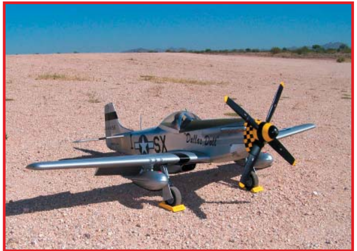
Cory Dale's immaculate P-51D. This started out as a 56" wingspan Kyosho ARF. Cory peeled it, made a new cowl, belly scoop, & drop tanks, with fiberglass and paint. It flies as good as it looks on glow.
