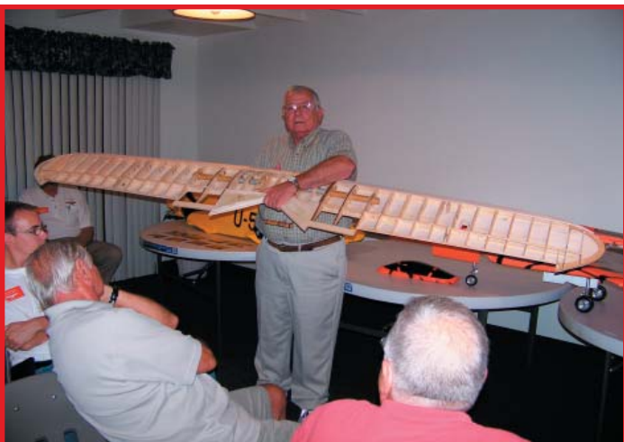
Rich Koehrer and his Staucher wing. Rich was surprised how large this small plane was after he finished the wing. Rich is selecting a power plant now.
