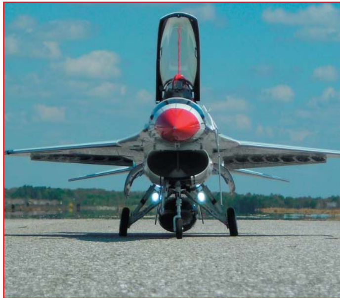
Luis Ceja, Top Gun Competitor's Avonds 1:6.9 Scale with a 44" wingspan. Powered with a jet cat P160 Turbine. (36 lbs Thrust) Take Off weight 34 lbs. Full cockpit, sliding canopy, smoke and built from USAF Thunderbirds #5 now flown by a pilot named Samantha. definitely not an ARF!
