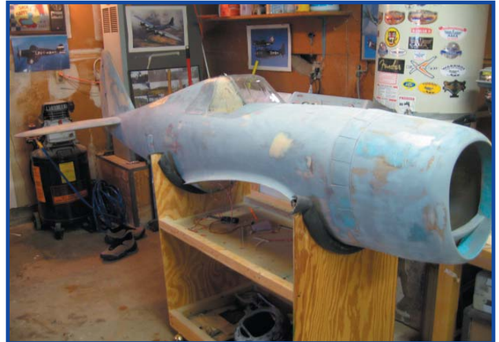
Brian Youngs huge Don Smith P-47 after a lot of glass and sanding prior to applying the panel lines.
