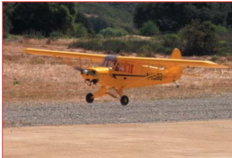
Gary Simlar's 106" wingspan Dave Patrick Cub with a Zenoah G26. The Prop is a 17 x 6 APC Gary is using a 2S2P 5200 Mah lion rx battery with a voltage regulator and an AR9000 receiver with two satellite receivers.
