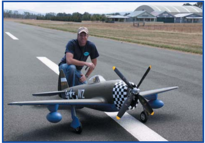
Greg Tracey in Australia and his new 92" wingspan all composite Robart ARF P-47 jug from a Nick Zirola design. It comes out of the box like that and you have several choices of paint schemes. Powered with a Zenoah G62. Set up for Robart air retract system and wheels.
