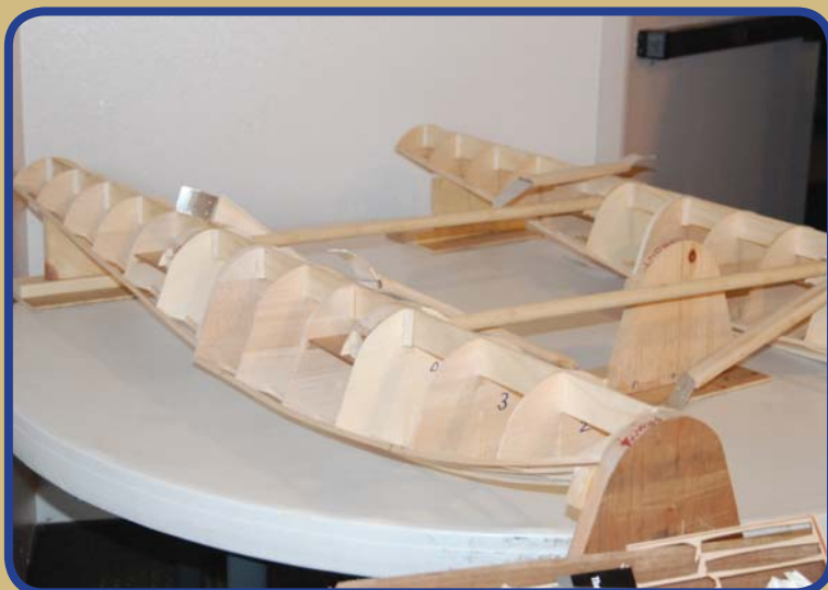
Larry Klingberg displays his new pontoons under partial construction. Larry has developed a mold system that ensures that both pontoons are exactly the same size.
