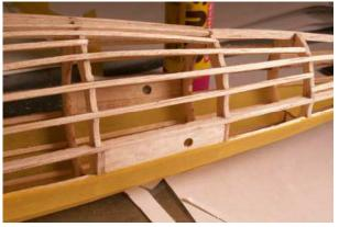
the fuselage. Sand flush to give a smooth seam.
