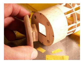
The removable nose block seen here with our Moses Magnets used to hold it secure in place.
