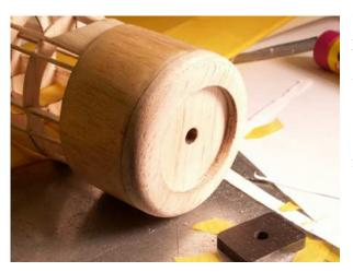
The removable nose block is then put in position and final sanding done to make sure the edges match perfectly. I'll add the nose button and prop only after I've got the plane gliding real nice. It keeps it lighter and will have the lowest drag for the best glide possible by your model.
