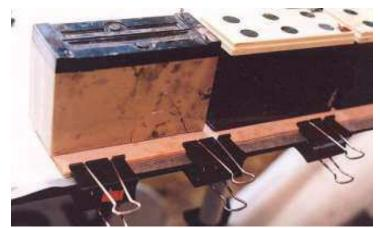
Brush epoxy finishing resin onto the 1/64" ply flap skins. Stack the skins and core on a layer of wax paper. Weight and clamp while the resin sets. This also seals the hinges inside. Another option is to clamp the assembly to a glass pane. Glass panes are very flat.
