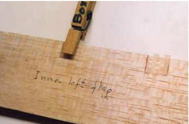
Remove and oil the brass hinge pins to prevent glue sticking to the pins. Glue the flap hinges to the balsa core.
