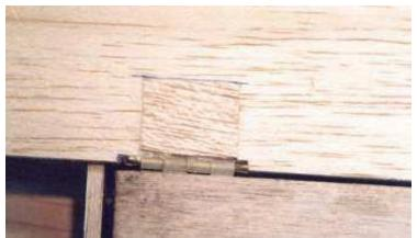
Cover the flap hinge's outer surface with 1/32" sheet balsa. Sand smooth.
