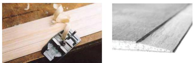
Start by cutting the layers of balsa and ply per the plans. Bevel the flap core trailing edge. Note that the upper ply layer is slightly shorter in chord. This allows the final result to have a tapered trailing edge.
