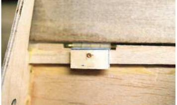
Install the flap strip on the wing. Pin the flap hinge to the spar with a lite-ply backing.
