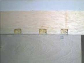
Rout hinge slots in a strip of wing sheeting. Reinstall the hinges and pins. Glue the forward half of the flap hinges to this strip.
