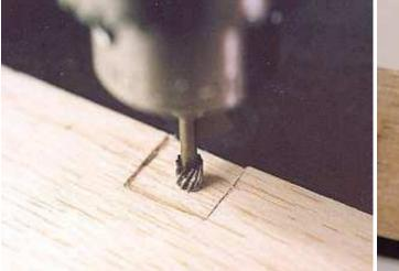
Rout out the balsa flap core 1/32" for hinges.
