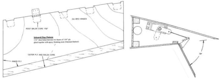
Split flaps on giant scale airplanes must be flat, stiff, light and strong. The method shown here achieves this by sandwiching a 3/32" balsa sheet core between two layers of 1/64" ply. These layers are glued together with finishing resin—a technique I learned from Roy Maynard. The result is light yet rigid.
