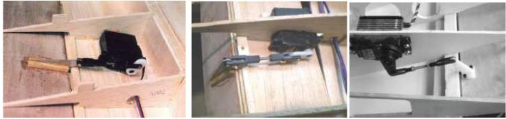
Install and test the flap horn and servo before sheeting the upper wing surface. Place the horn over a hinge to minimize bending of the flap during movement. For large flaps, a bolt-on horn is recommended.
