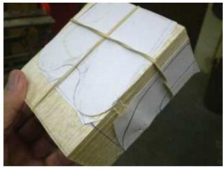
Cut the top view with a scroll saw or bandsaw and spot-glue the pieces back in place.
