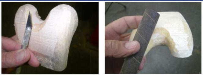
Round the edges using an X-Acto knife, sanding spindle tube, sanding block and sandpaper,
