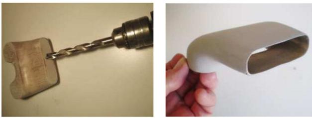
Sand the surface. Drill out the balsa core. Continue removing the core with an X-Acto knife, file, sandpaper etc, leaving nothing but the fiberglass covering. This is known as the "lost wax" method.
