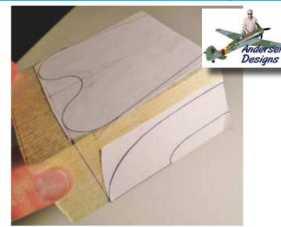
Apply the top view and side view onto a balsa block.
