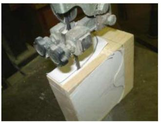
Cut the side view with a bandsaw.
