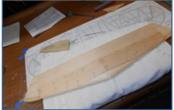
Photo 11: Elevator outside edges presented some challenges due to some odd gaps & dips.
