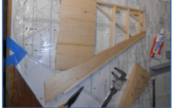
Photo 16: Fitting the rudder to the fin turned out to be a bit anticlimactic. Here everything is ready for hinges.
