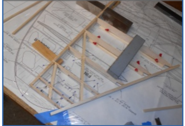
Photo 15: Fin sheeted, completed & ready for finish sanding.
