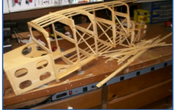
Photo 6: Stringers & longerons are removed leaving the cabin and engine compartment.
