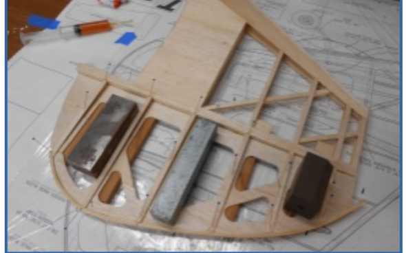
Photo 16: Fitting the rudder to the fin turned out to be a bit anticlimactic. Here everything is ready for hinges.
