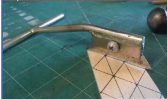
Photo 3: The Chopper set up to mass produce as many 45° angle gussets as any modeler can wish for.
