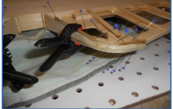
Photo 12: Completed stab ready for hinges.
