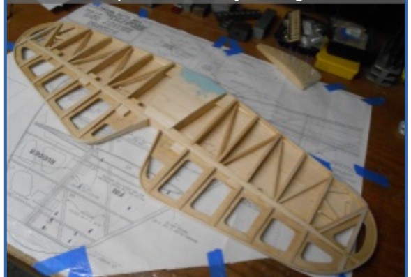
Photo 12: Completed stab ready for hinges.
