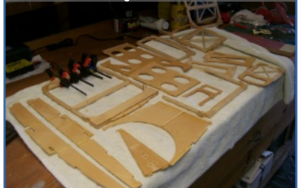
Photo 8: Parts & subassemblies that will be used to reconstruct the fuselage.
