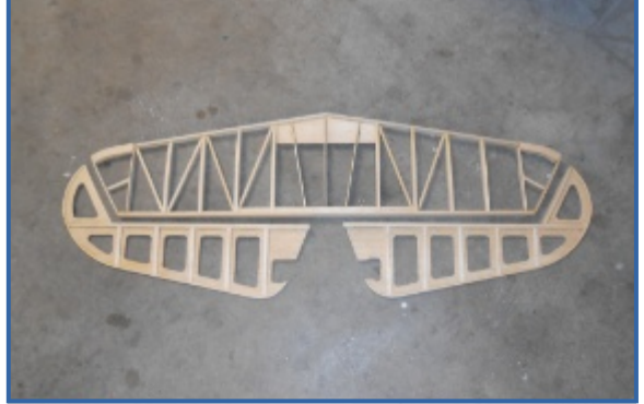
Photo 10: Sheeting completed on the bottom of the stab.
