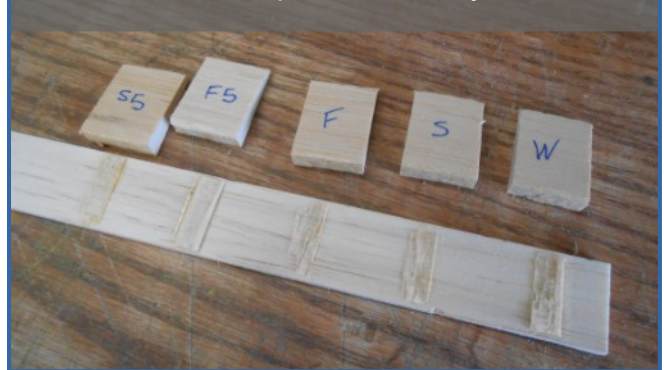
Photo 5: All joints held very well with no discernable difference in the force required to break the joints.
