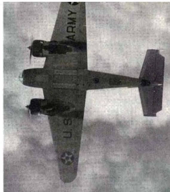
Under-wing lettering for most trainers was 24 inches tall. Though the above photo clearly shows the angled corners of the letters, there were times when the lettering was rounded by manufacturers.
