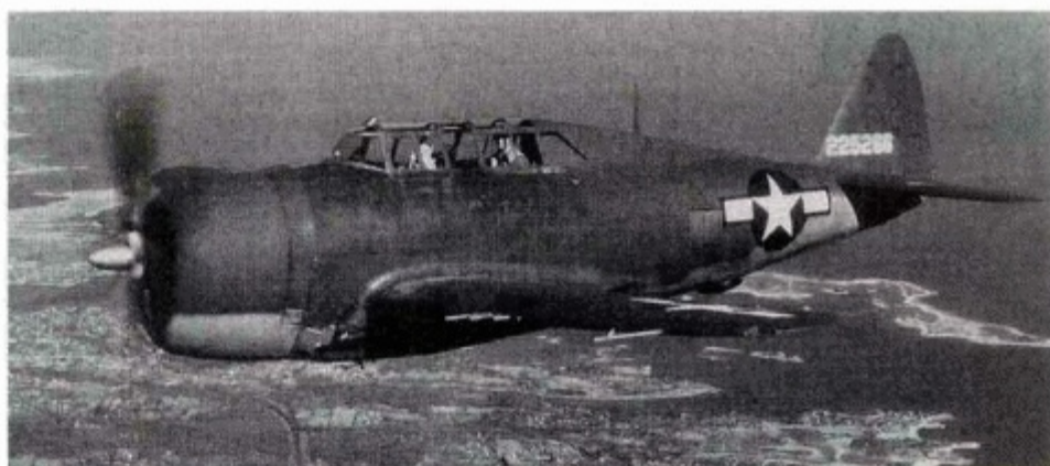
A rare Republic TP-47G Thunderbolt (two-place trainer version) is dressed with the blue-and-white star-and-bars insignia. The overall finish is olive drab with a neutral gray underside.
