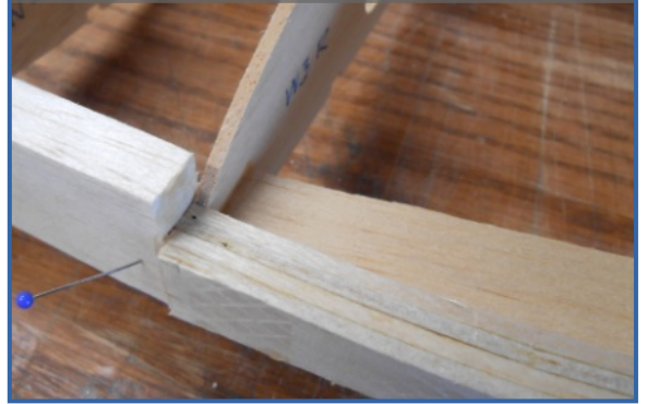
Photo 4: Wing tube guides ready for installation in the wing panels.
