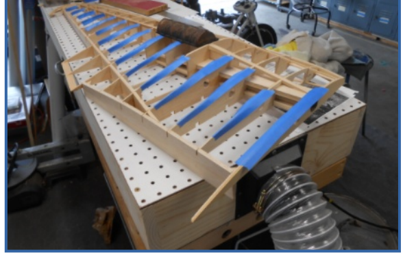
Photo 8: Sheeting the inner top of the leading edge. At this point, the sheeting is shaped and glued only to the leading edge. The spring clamps force the rest of the sheet into a curve that will be easier to glue as a second step.
