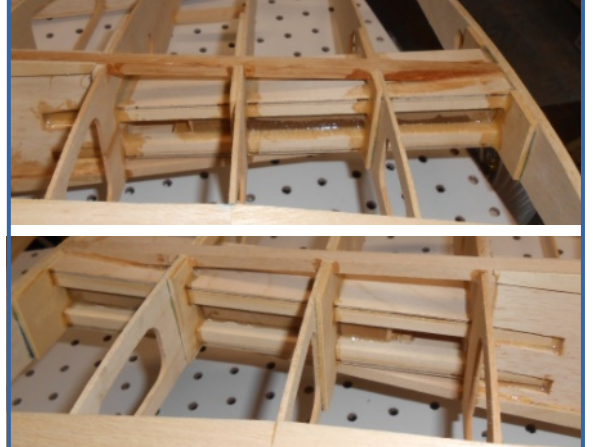
Photo 6: Here's the best I could do with epoxy & an acid brush (upper photo) vs. using a regular glue syringe (lower).
