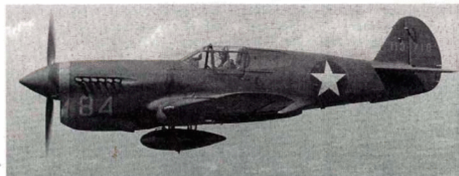
Here, an all olive drab P-40 wears the star-and-blue-circle insignia with red center painted over. The nose and tail numbers were probably yellow. In May 1942, for air operations in North Africa, olive drab finishes were replaced with Desert Sand FS 30279. The neutral gray underside was also replaced with Azure Blue FS 35231.
