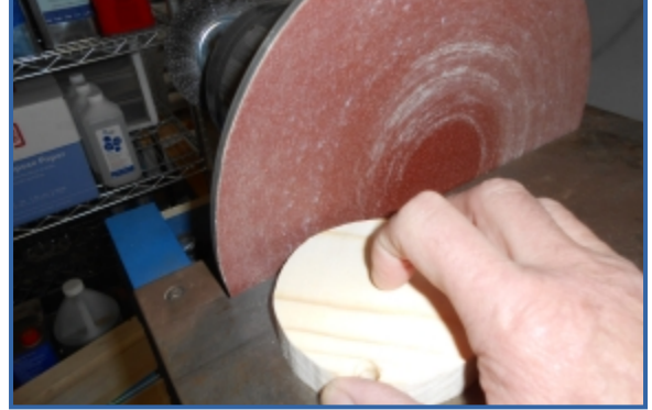
Photo 10: Parts to plug the dead end of the drain pipe.
