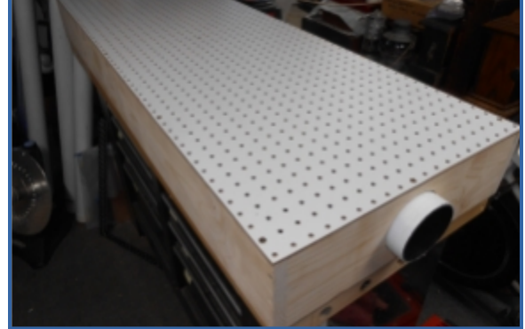
Photo 14: Surface-mount inlet flange used to replace drain pipe nipple that was too big.
