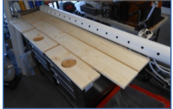
Photo 6: Front board attached to end using carpenter's glue and drywall screws.
