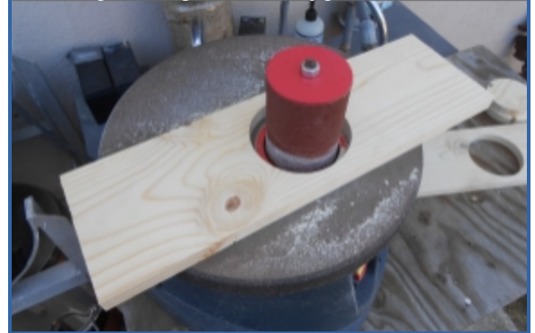
Photo 4: Truing up the 4" holes in the crosspieces after rough-cutting them with a jigsaw.
