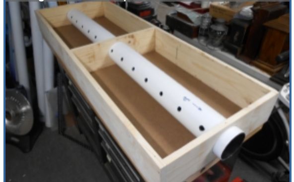
Photo 12: Table bottom and drain pipe installed and waiting for the table top.
