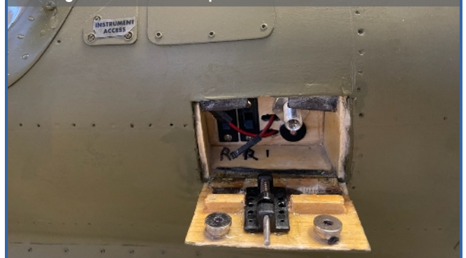
Photo 4: Service bay containing charging cables, switches & air filling connector for the pneumatic retracts.
