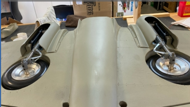
Photo 8: Retracts look like they were made for the model... because they were.
