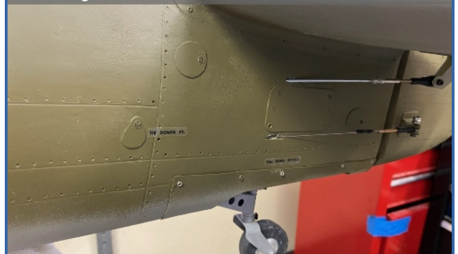
Photo 4: Service bay containing charging cables, switches & air filling connector for the pneumatic retracts.
