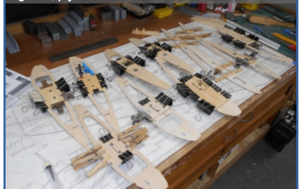
Photo 4: After gluing the balsa parts of the ribs together, plywood doublers are added.
