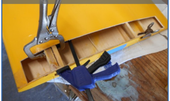
Photo 6: Reattaching the end rib to the right wing panel.
