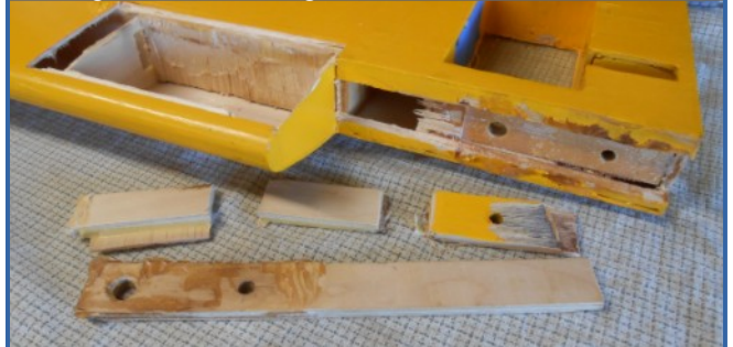
Photo 2: After opening the bottom wing sheeting I was able to wrestle the remains of the spar out of the wing without causing even more damage.
