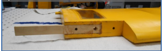
Photo 2: After opening the bottom wing sheeting I was able to wrestle the remains of the spar out of the wing without causing even more damage.
