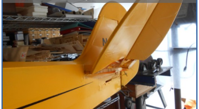
Photo 7: Horizontal and vertical stab braces were never installed. It's a wonder only one side of the stab broke off.
