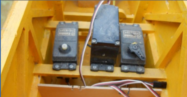
Photo 16: Interesting servo installation. That inverted one is for throttle. These are all giant-size servos that were popular during the 1990s.
