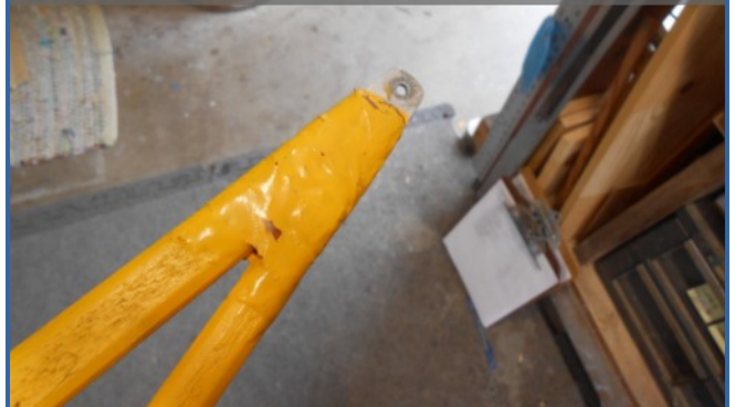
Photo 7: Horizontal and vertical stab braces were never installed. It's a wonder only one side of the stab broke off.
