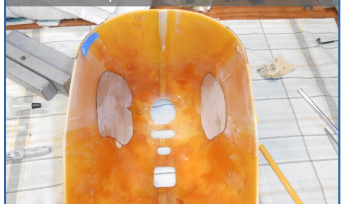
Photo 4: The 1/64" patches installed on the inside of the cowl.
