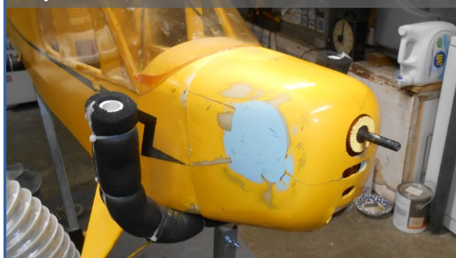
Photo 8: Blue tape showing where the split line will be. This will allow the cowl to be removed without having to dismantle the engine.
