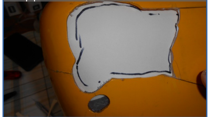
Photo 3: Templates & patches ready to be epoxied in place.
