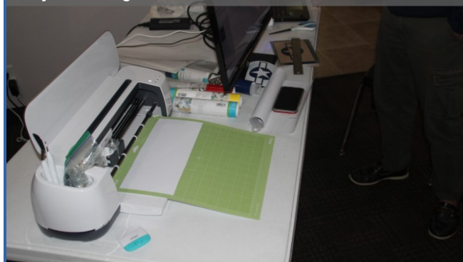
Photo 5: A piece of white vinyl attached to a backing board, ready for cutting.
