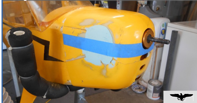
Photo 8: Blue tape showing where the split line will be. This will allow the cowl to be removed without having to dismantle the engine.
