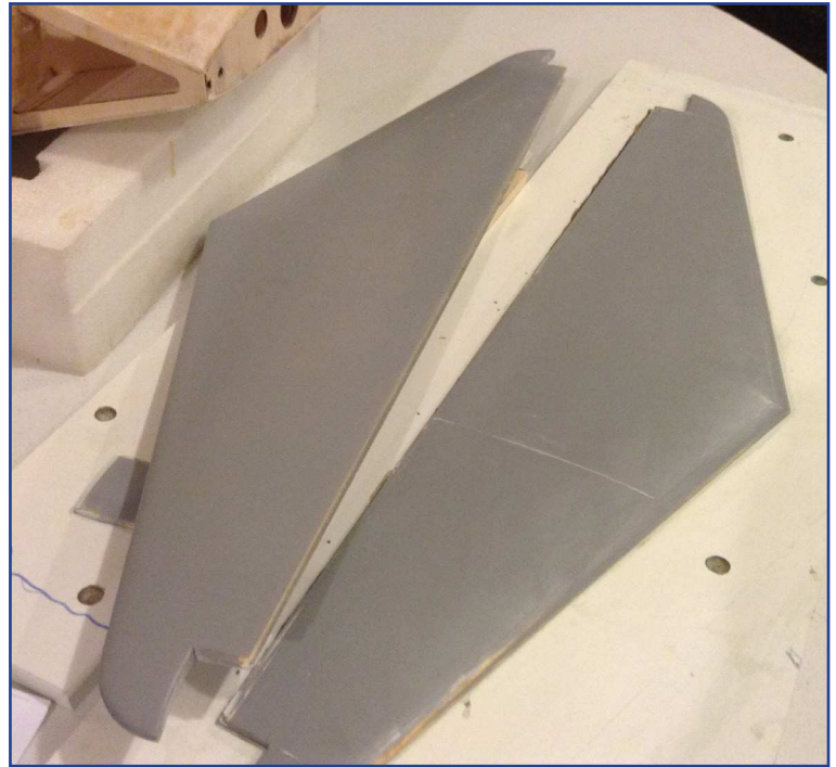
A photo of the horizontal stab plug (left) and the actual vacuum bag part on the right. The stab features all the panel lines. The entire project has been scaled exactly to the full size Panther at the Yanks Air Museum
