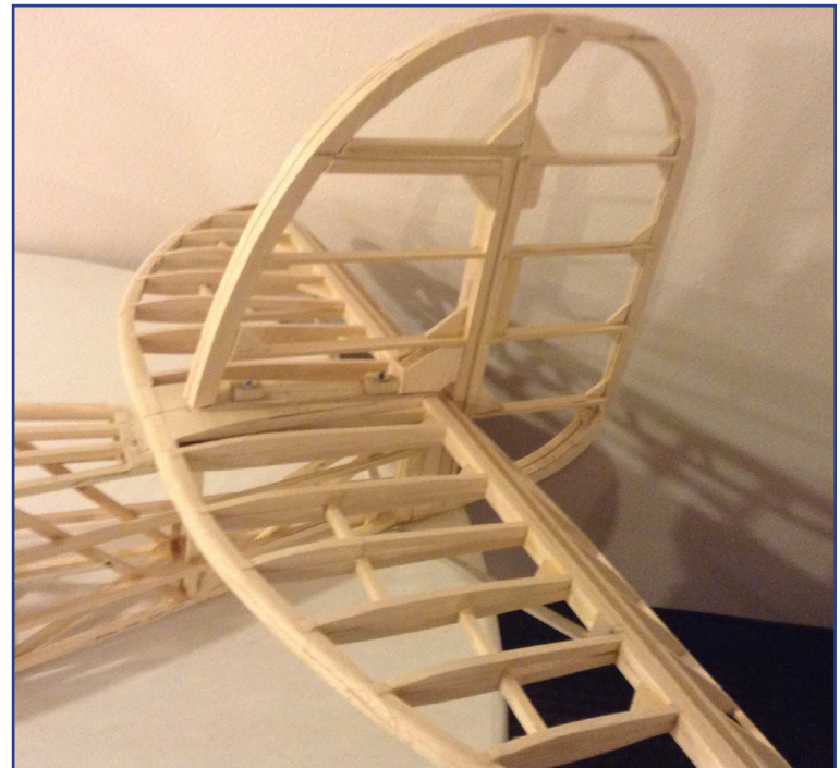
A good close up of Larry's construction for the tail group. Larry cuts the wood and works from plans and sometimes sketches since a lot of the information and documentation is not available.
