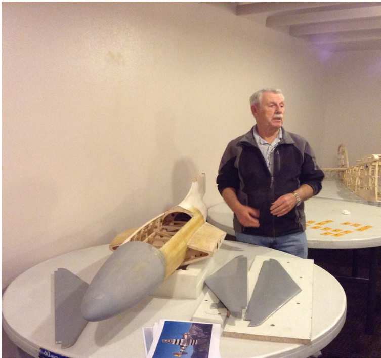
Larry Wolfe shows the progress on a joint project he and Sam Wright tackled. A 72" F9F Panther. This is the start of the fuselage plug. The Panther will be set up for EDF (Electric Ducted Fan) Turbines can be installed as well with the correct plumbing.
