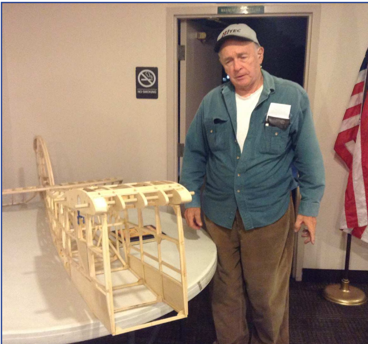
Larry Klingberg shows his latest all scratch built project. This is a 1/3rd scale Fairchild FC2. Built in 1927 and has a 12' wingspan. Larry's work is really too nice to cover up!
