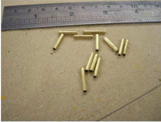
The tube cut ready to thread onto the wire hinge pin. (see next Photo)
