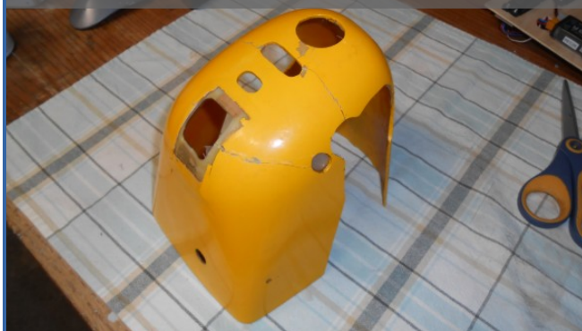
Photo 4: All the big pieces reassembled. Note the huge gap in the side. I'll come back to that in a minute.
