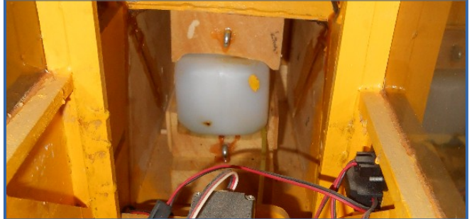
Photo 8: Looking into the fuselage from the trailing edge of the wing you can see the fuel tank held in place with two giant balsa blocks. This made it impossible to access the back of the firewall.
