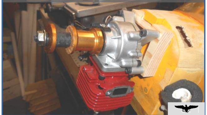
Photo 12: This is the side where the Pitts-style muffler will be attached. There's no chance I'll be able to hide that.
