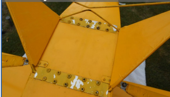
Photo 2: Six LG straps and 12 machine screws will make maintenance much easier. The little white dots are the filled holes where the machine screws used to live.
